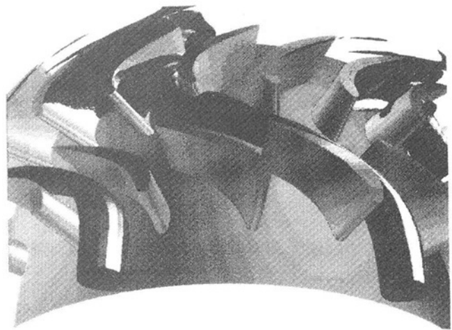
Fig. 16 Snapshot in time of three-dimensional unsteady Euler simulation of hot streak in LSRR stage turbine. The hot streak convects through the stator passage with no distortion and then interacts with the passing rotor.
